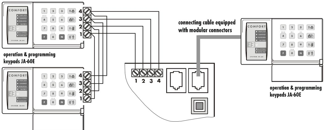
When a control panel has a JA-65R radio communicating module installed, it can also be operated and programmed via JA-60F wireless keypad(s) asunder this situation, a minimum of one JA-60E keypad should be connected to the control panel. With a 65R module, the system can also be operated by remote controls RC-11, RC-22 & RC-60, as well as by a JA-60D wireless keypad. The control panel can have up to 8 wireless controllers.
